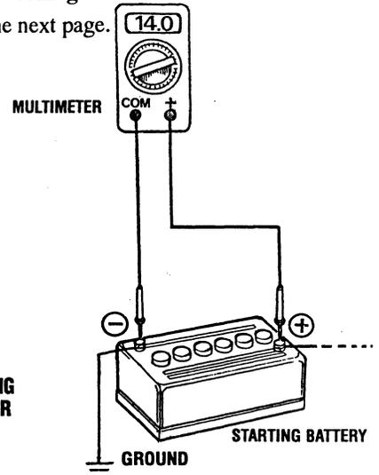
TESTING THE STARTING BATTERY-ALTERNATOR (ENGINE RUNNING)
