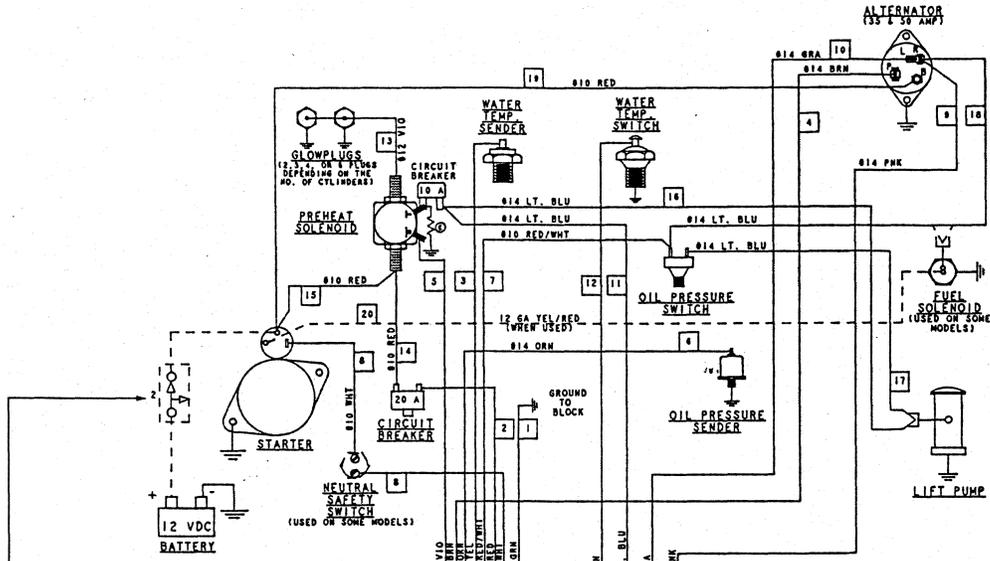
**NOTE :** An on-off switch should be installed in this circuit to disconnect the starter from the battery in an emergency and when leaving the boat. Twelve volt diesel engine starters typically draw 200 to 300 amps when cranking. A switch with a continuous rating of 175 amps at 12 VDC will normally serve this function, but a switch must never be used to "make" the starter circuit.
