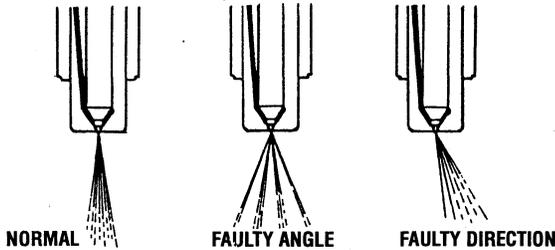
2. Apply the pressure of 115 kg/cm<sup>2</sup> (1635 lb/in<sup>2</sup>) to nozzle by operating the hand lever, and check the drips from the nozzle tip. If it drips or has a large accumulation of fuel on the bottom, it is considered defective and should be replaced. A very small amount of fuel may sometimes remain on the tip of the nozzle; however, this does not indicate a defect.
