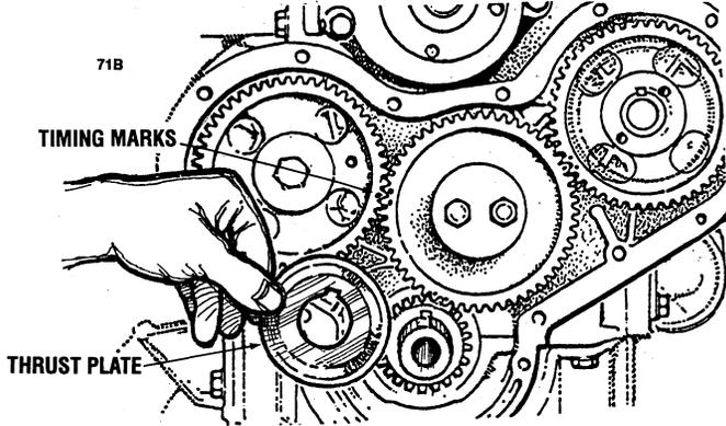
10. Install each gear. While aligning the timing mark of each gear, install the following gears on each position.
