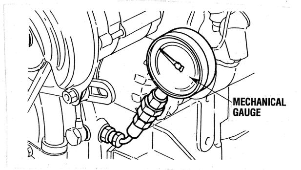
**⚠ CAUTION: Oil Pressure Switch - Do not use lock pliers, vise grips or pipe wrenches on the oil pressure switch. Use the correct socket which is available from Snap-On, Proto, New Britain and others. Damage to the switch will cause oil leaks and/or switch failure.**
