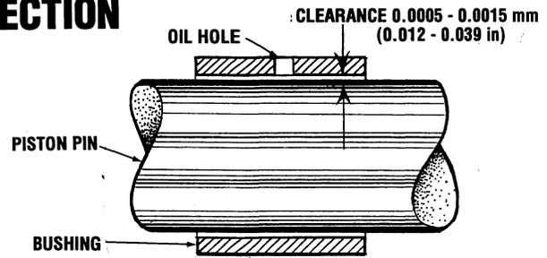
**4. Small end bushing replacement.** Using a press, press out the bushing. Align the oil passages of the connecting rod and the small end bushing; press in the bushing to the connecting rod bore. After a small end bushing has been replaced, ream the bushing bore to obtain the specified clearance between the small end bushing and the piston pin.
