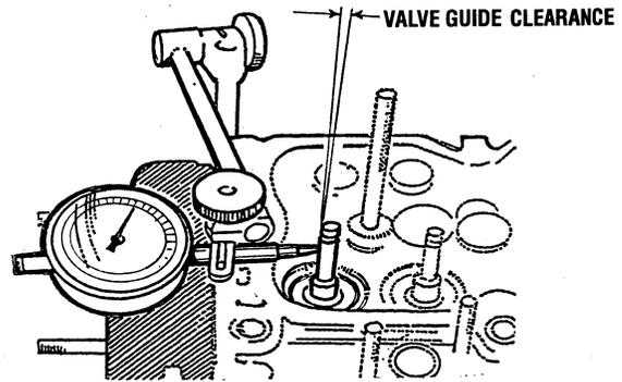
**2. Valve guide replacement.** To remove the valve guide, press out the valve guide towards the combustion chamber side, using the valve guide installer (49 0636 165A). Again using the valve guide installer, press in the valve guide into the cylinder head until the valve guide height reaches the indicated scale on the valve guide installer.
