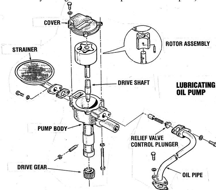
2. Clearance between pump body and shaft. Measure the above clearance with a dial gauge and magnet base.
