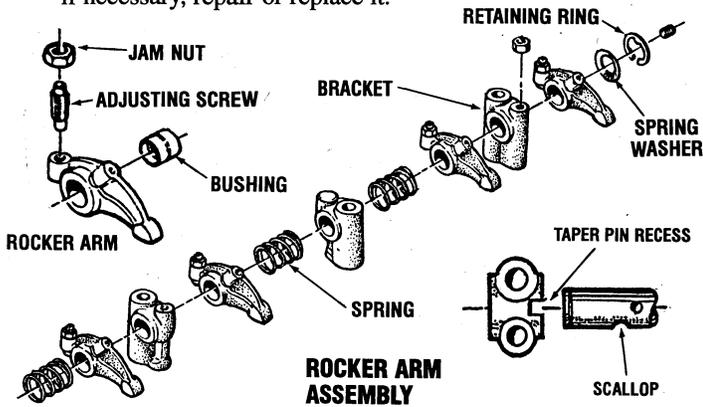
**2. Inspecting clearance between rocker arm and shaft.** Check the clearance between the rocker arm and shaft and, if it exceeds the limit, replace the rocker arm bushing or shaft.
