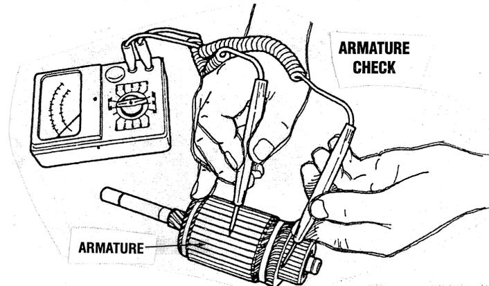
2. Measure the commutator O.D. and the depth of undercut. Repair or replace it if the service limit is exceeded. Also check the commutator outside surface for dirtiness and roughness. If rough, polish the commutator with fine crocus cloth.
