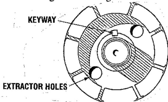
**NOTE:** If an extractor is not available, replace the nut on the injection pump shaft loosely and with a nylon drift and hammer gently tap the injection pump shaft to dislodge it from the keyed drive gear.
