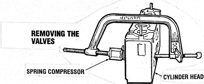
36. Remove each valve from the cylinder head assembly. Use an appropriate valve spring compressor to aid in disassembly. Arrange or label valves so as to replace them in the cylinder and the guide from which they were removed.
