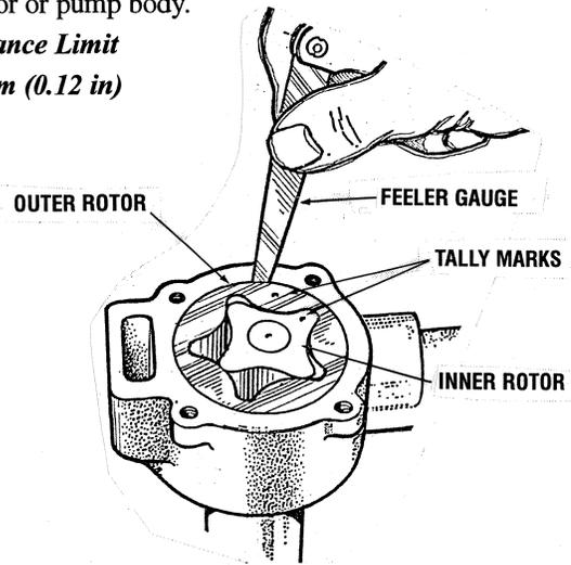
5. Clearance between rotor and pump cover. Check the end float of the rotors. Place a straight edge across the pump body and measure the clearance between the rotor and straight edge with a feeler gauge. If the clearance exceeds the limit, replace the drive gear, drive shaft, inner rotor, outer rotor and pump body.
