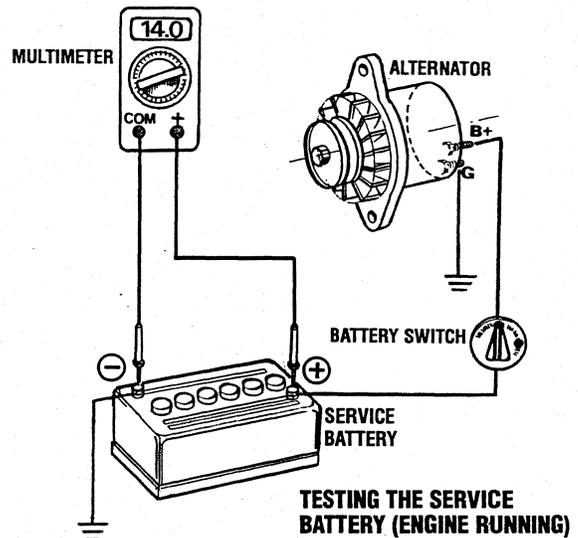
**CAUTION:** When performing tests on the alternator charging circuit do not use a high voltage tester (i.e. Megger). You can damage the alternator diodes.
