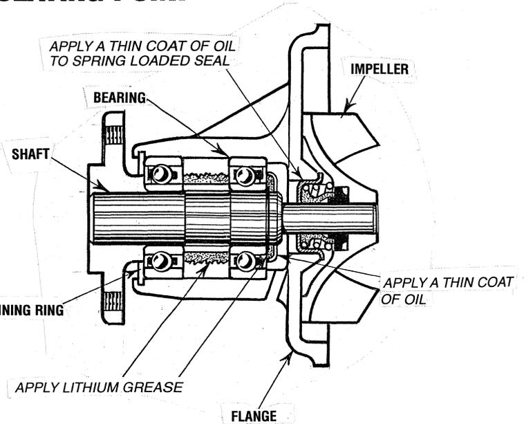
**NOTE:** Do not allow oil or grease to contaminate the surfaces of the ceramic ring or the graphite (small end) of the spring-loaded seal.
