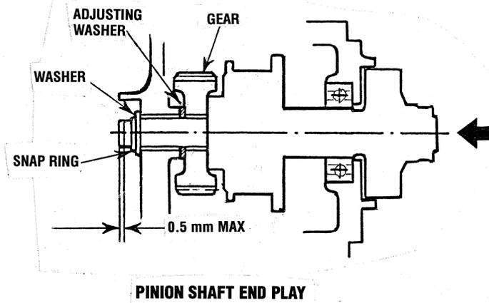
Reassemble the starter assembly in the reverse order of disassembly, making sure of the following:
