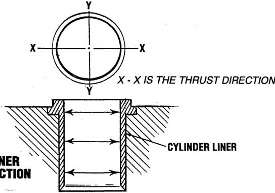
**CYLINDER LINER WEAR INSPECTION**
