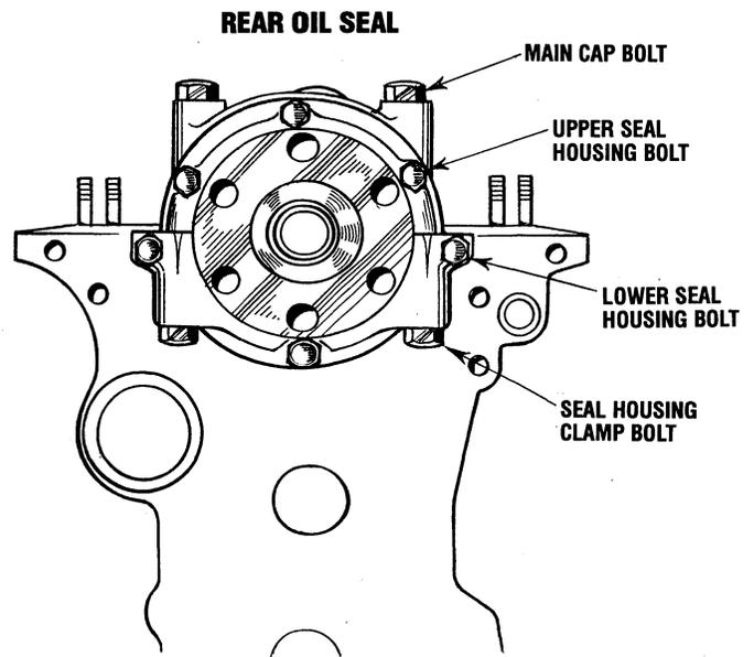
**3. To refit the assembly:** Thoroughly clean the butt joint between the half-housings.
