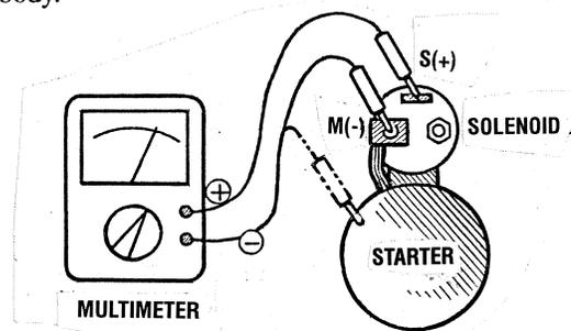
**NOTE:** Disconnect the wire from terminal M.
