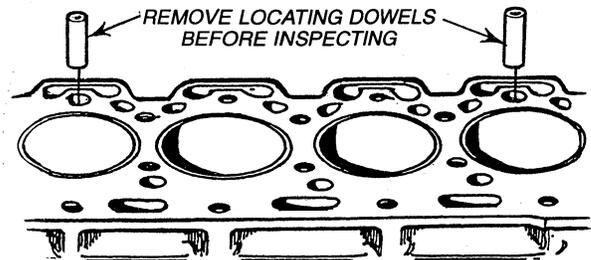
**2. Distortion Inspection.** Check the gasket face distortion of the cylinder block and if it exceeds the limit, repair or replace it.
