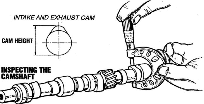
**3. Inspecting camshaft journal.** Check the camshaft journal and, if wearing exceeds the limit, replace the camshaft.
