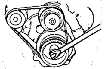
REMOVING THE CRANKSHAFT PULLEY
