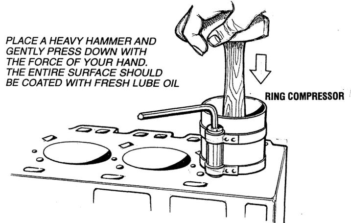
**INSTALLING PISTON AND CONNECTING ROD ASSEMBLY**
