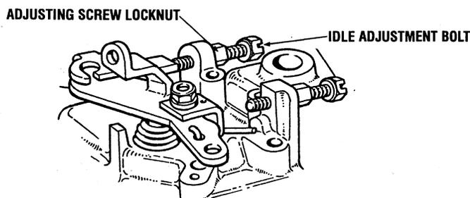
3. Inspecting and adjusting the injection pump timing.
